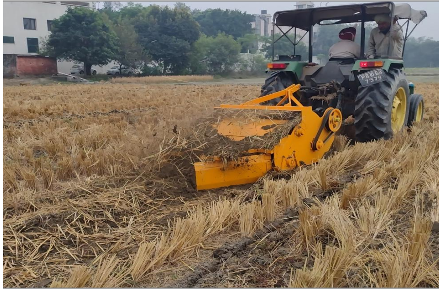
Fig. 2: Working view of tractor-operated bund former
