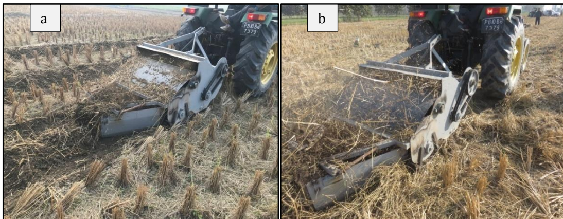
Fig. 3: Working view of tractor-operated bund former in field under straw load (a) 4.0-4.5 t.ha -1 , and (b) 6.0-6.5 t.ha -1
