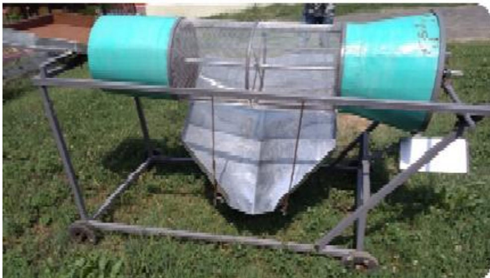
Fig. 3: Developed earthworm-cum-compost separator
