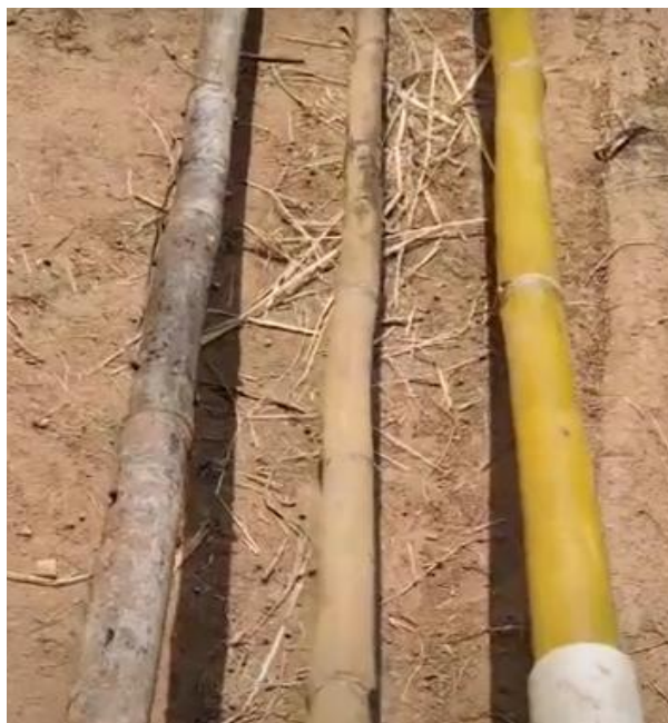
Fig. 2: Difference between 1) non-treated bamboo, 2) treated bamboo, and 3) treated bamboo with polish
