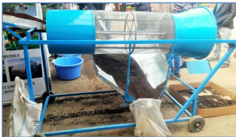
Fig. 4: Evaluation of earthworm-cum-compost separator
