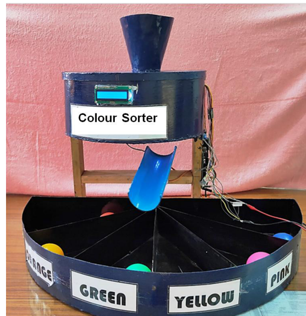
Fig. 6: Sensor-based automatic colour sorting system
